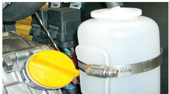
Coolant Bottle Replacement
