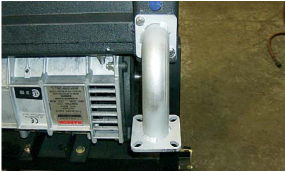
Frame Flange Replacement
