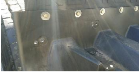
Rear fairing mounting holes are moved out 1" in mud flap holder.
