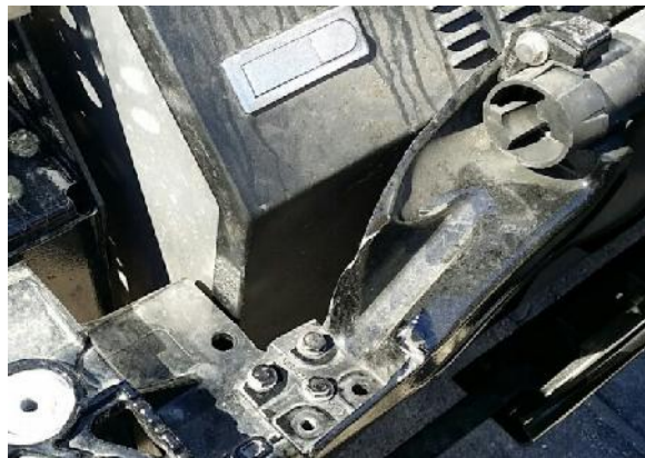
1" spacers are inserted between bracket and fairing. (Brace is left in original position at frame.)
