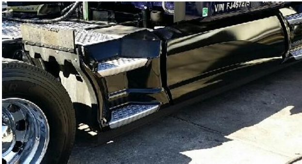
Finished installation with usable stels Both fairings moved out 1" and it's virtually undetectable.
