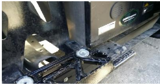
Lower fairing bracket trimmed
