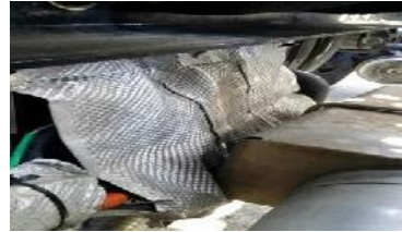
Heat shielding. Driver still plans to move exhaust away from APU with an "S" curve.
