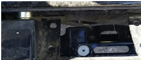
1" spacers are inserted between bracket and fairing. (Brace is left in original position at frame.)
