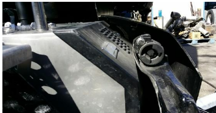
Lower fairing bracket trimmed
