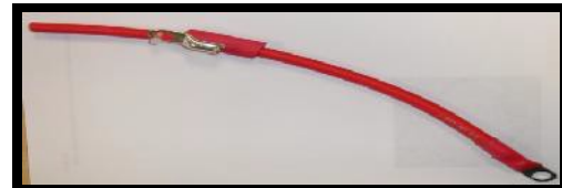
54-8204 E - Fuse Block to Battery Cable
