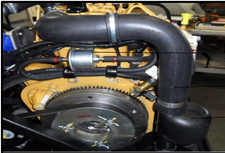
Fuel Pump, Hose, Intake hose, Resonator Assembly
