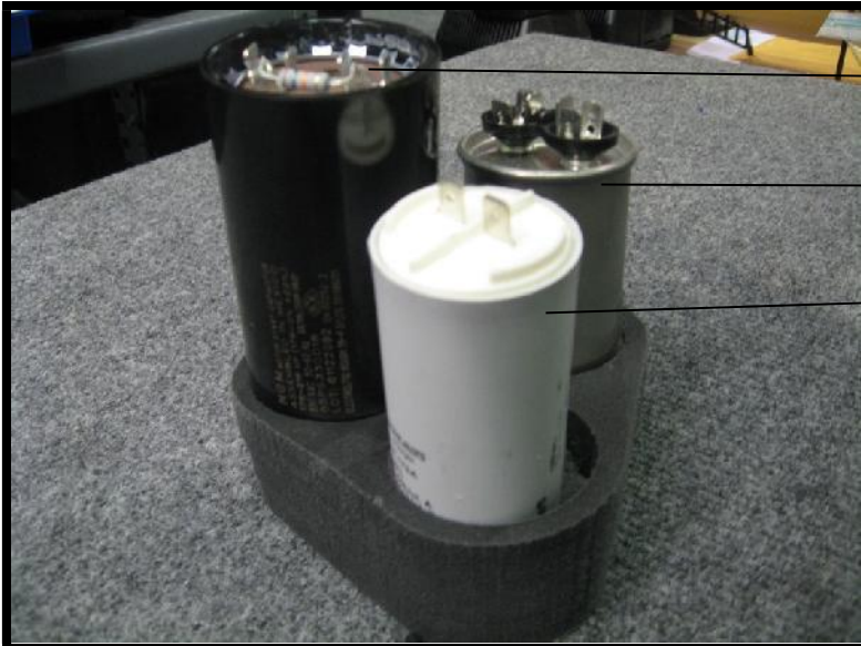
Compressor Start, Run Capacitor, Blower Motor Capacitor
