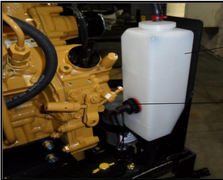
Coolant Recovery Bottle, Coolant Level sensor
