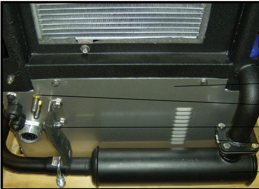
Intermediate pipe, hanger, muffler, panel, fuel ports
