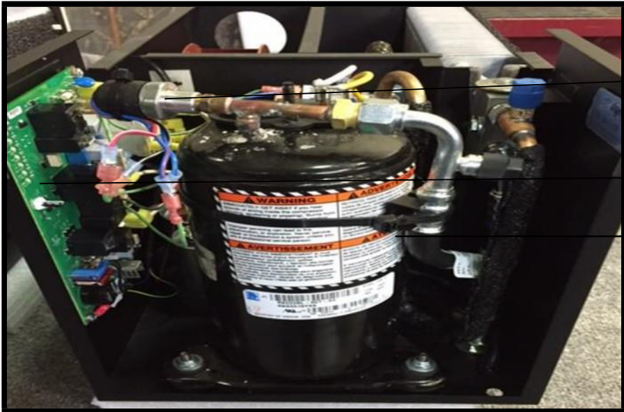
High Side Switch, #8 Discharge Hose, PCB Assembly
