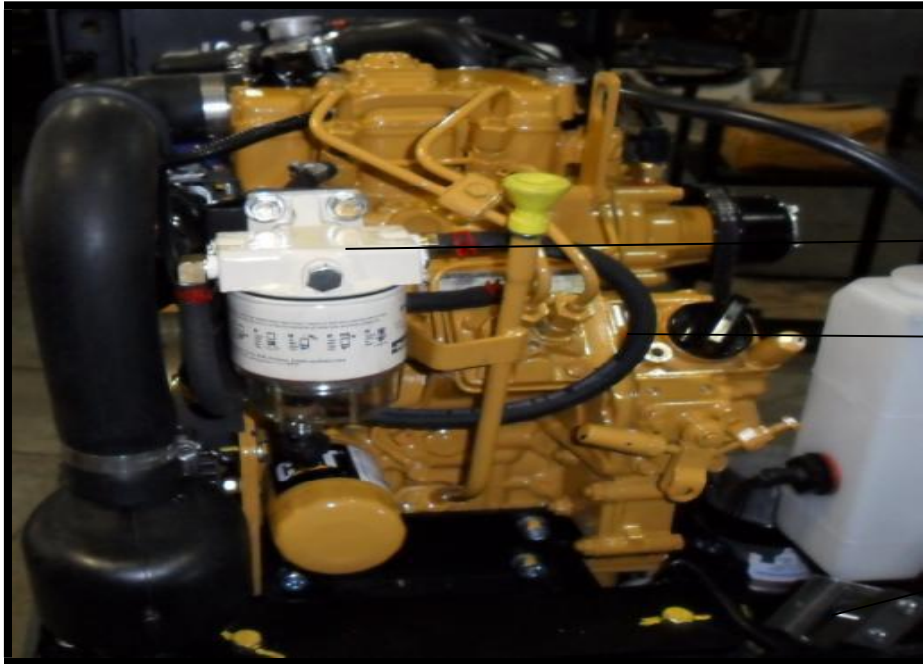
Fuel Filter / Water Separator Assembly, Safety Switch
