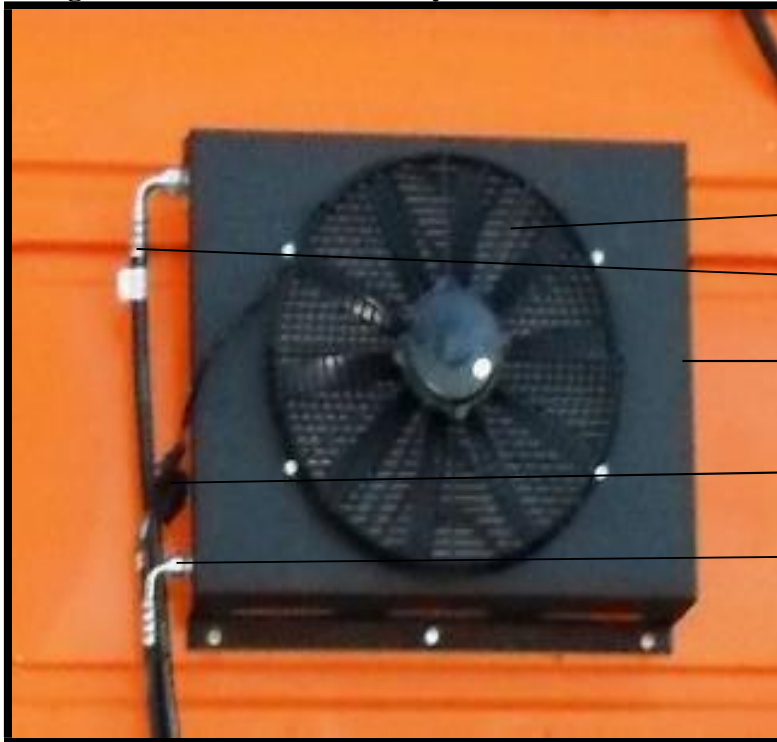
Integrated Condenser, Fan, Harness, Hoses, Shroud
