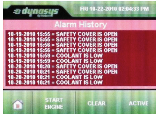
Figure 8 Alarm History Screen
